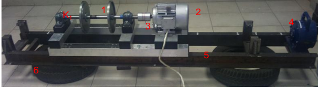
Fig. 2.1. Test stand: 1. two-disk rotor, 2. motor, 3. coupling, 4. indicator, 5. frame, 6. favourable ground
